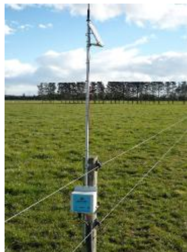
AQUACOM and AQUAFLEX Dairy Pasture Application with Radio Telemetry
